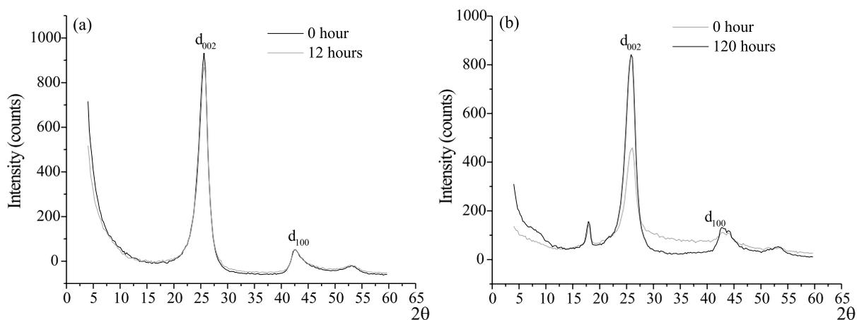
Fig. 5. Powder X-ray diffractograms before and after grinding for *thin* (a) and *thick* (b) nanotubes.
