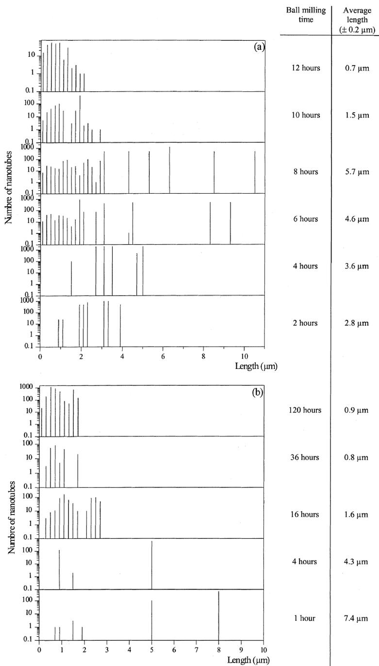
Fig. 2. Measured *thin* (a) or *thick* (b) length distribution of the nanotubes for different ball milling times.
