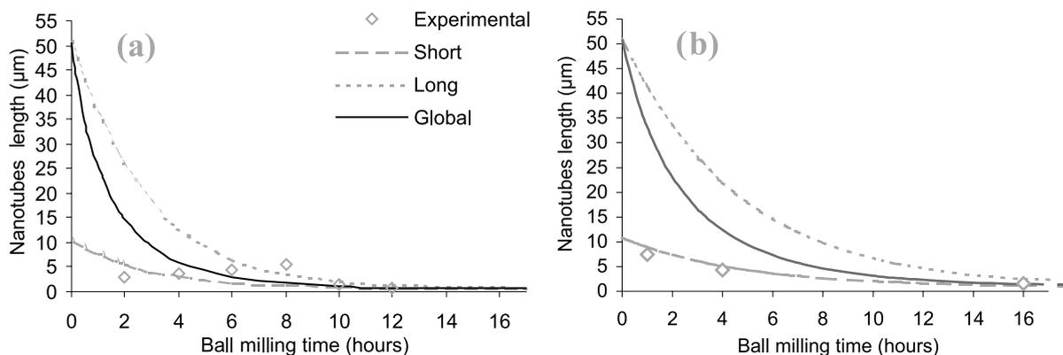
Fig. 4. Time evolution of carbon nanotube average length for *thin* (a) and *thick* (b) nanotubes.
