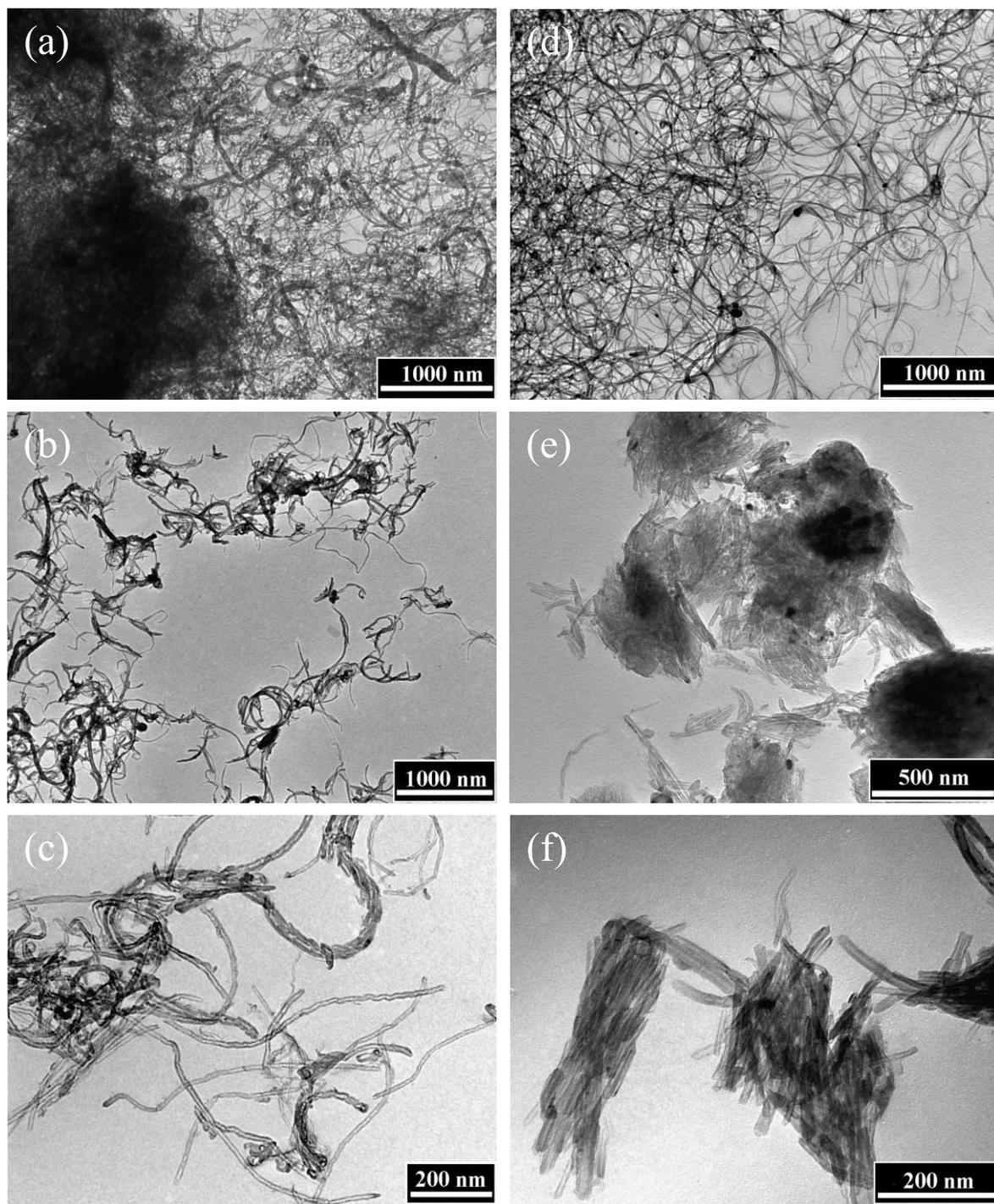
Fig. 1. Low magnification TEM images of multi-wall carbon nanotubes. (a–c) *Thin* nanotubes before (a) and after (b, c) 12 h of ball milling. (d–f) *Thick* nanotubes before (d) and after (e, f) 120 h of ball milling.
