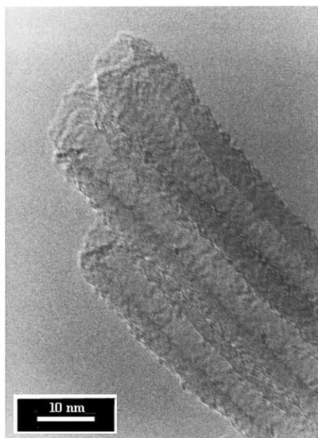
Fig. 3. HREM image of short *thick* carbon nanotubes after 120 h of ball milling.
