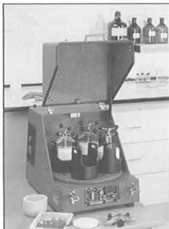
Fig. 1 Planetary Ball Mill „pulverisette 5“
