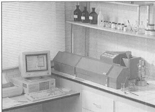
Fig. 2 Laser Particle Sizer „analysette 22“
