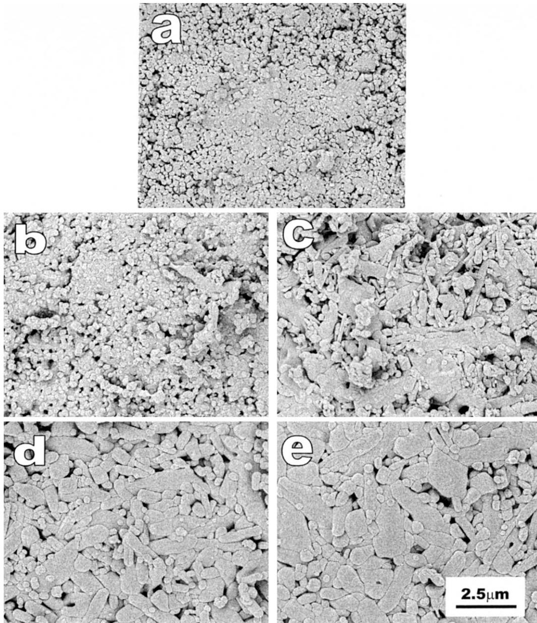
Fig. 5. SEM images of the  $\text{FeO}_{1.5}$ -doped mixture sintered at different temperatures: (a)  $1000^\circ\text{C}$ , (b)  $1100^\circ\text{C}$ , (c)  $1200^\circ\text{C}$ , (d)  $1300^\circ\text{C}$  and (e)  $1400^\circ\text{C}$ .
