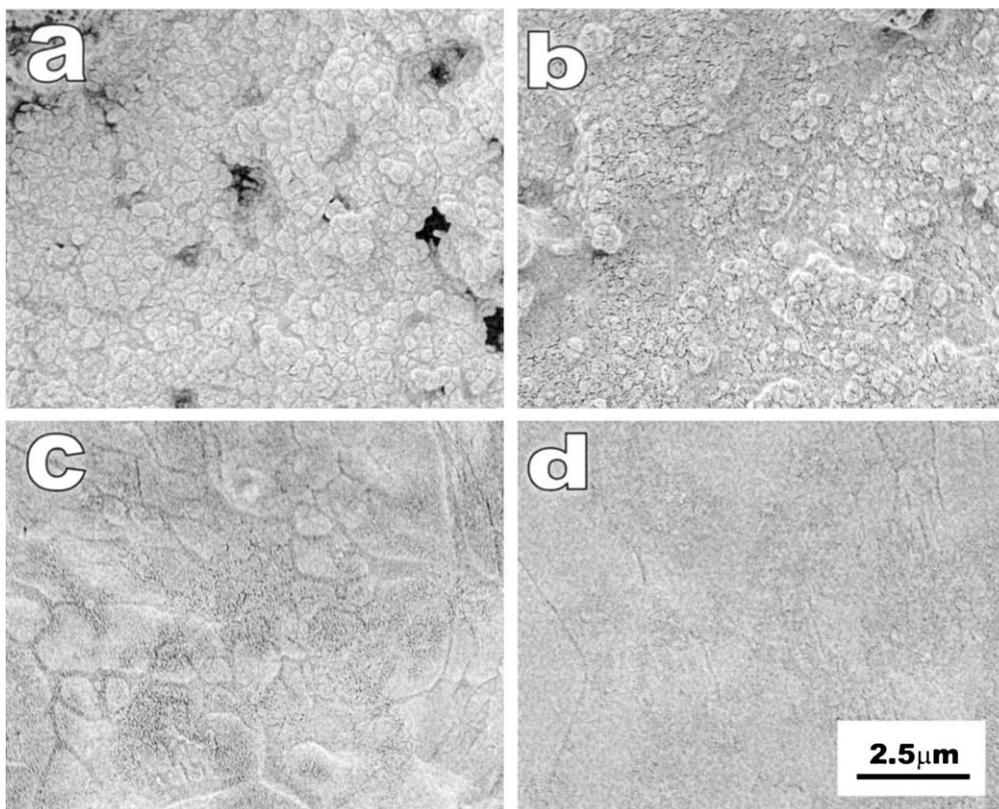
Fig. 8. SEM images of unmilled mixture of Al<sub>2</sub>O<sub>3</sub> and silica for pure mullite sintered at: (a) 1100 °C, (b) 1200 °C, (c) 1300 °C and (d) 1400 °C.
