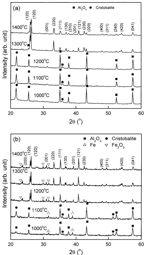
Fig. 3. XRD patterns of the undoped mixtures of  $\text{Al}_2\text{O}_3$  and silica for pure mullite sintered at different temperatures: (a) unmilled and (b) milled for 5 h.
