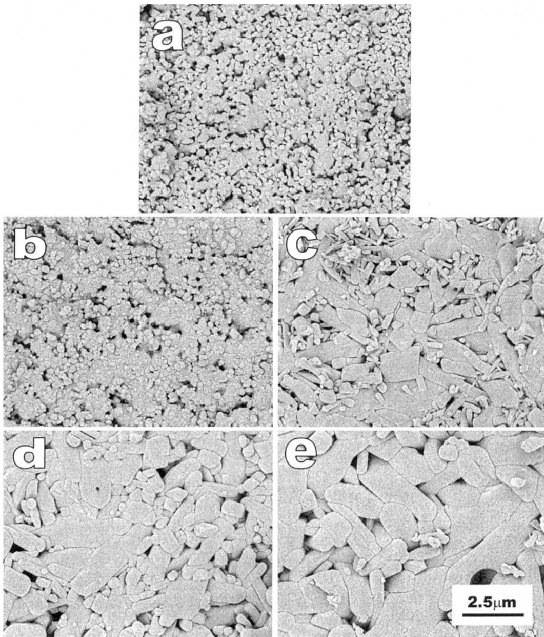
Fig. 6. SEM images of the CoO-doped mixture sintered at different temperatures: (a) 1000 °C, (b) 1100 °C, (c) 1200 °C, (d) 1300 °C and (e) 1400 °C.
