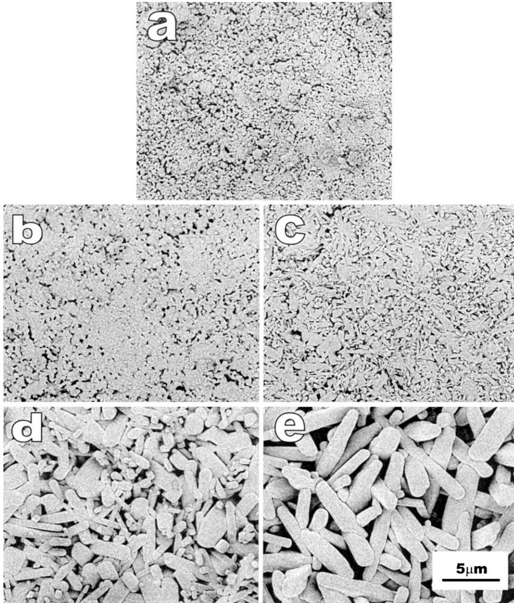
Fig. 9. SEM images of the milled mixture of  $\text{Al}_2\text{O}_3$  and silica for pure mullite sintered at: (a) 1100 °C, (b) 1200 °C, (c) 1300 °C and (d) 1400 °C.
