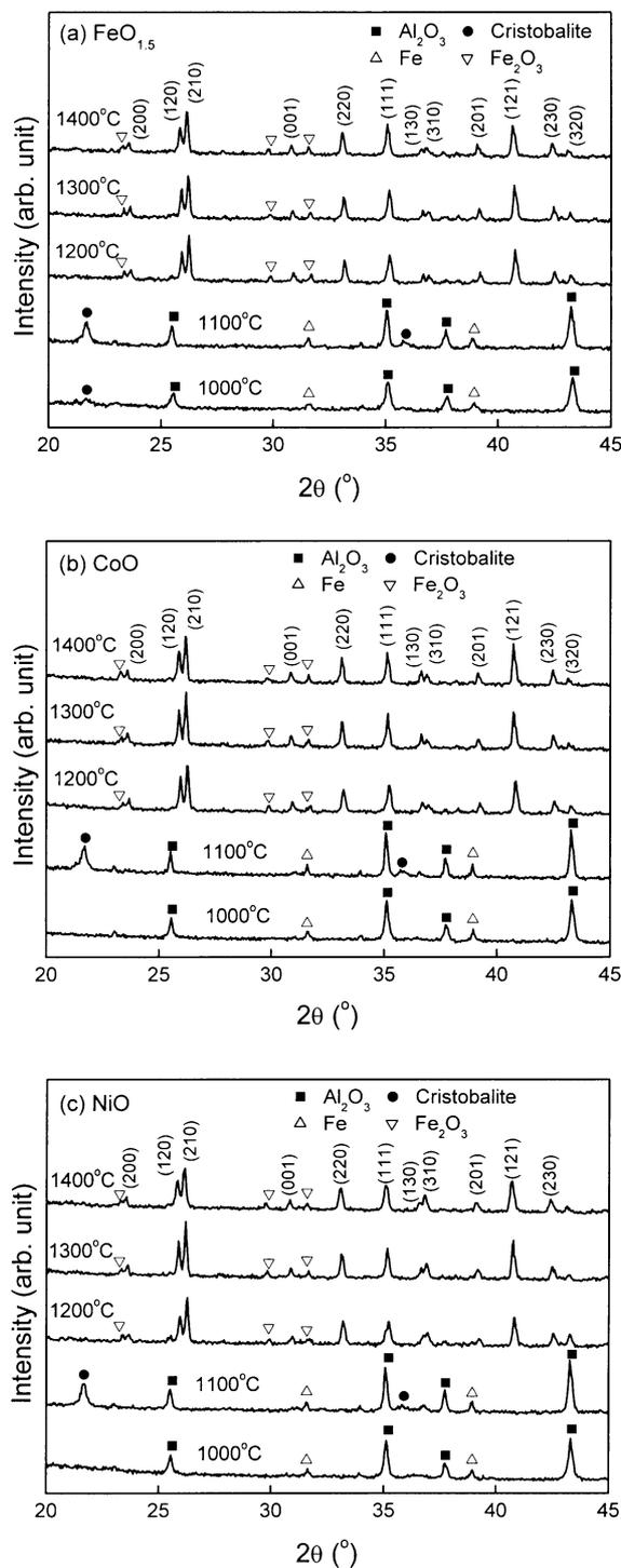
Fig. 2. XRD patterns of the milled mixtures doped with the transition metal oxides sintered at different temperatures.
