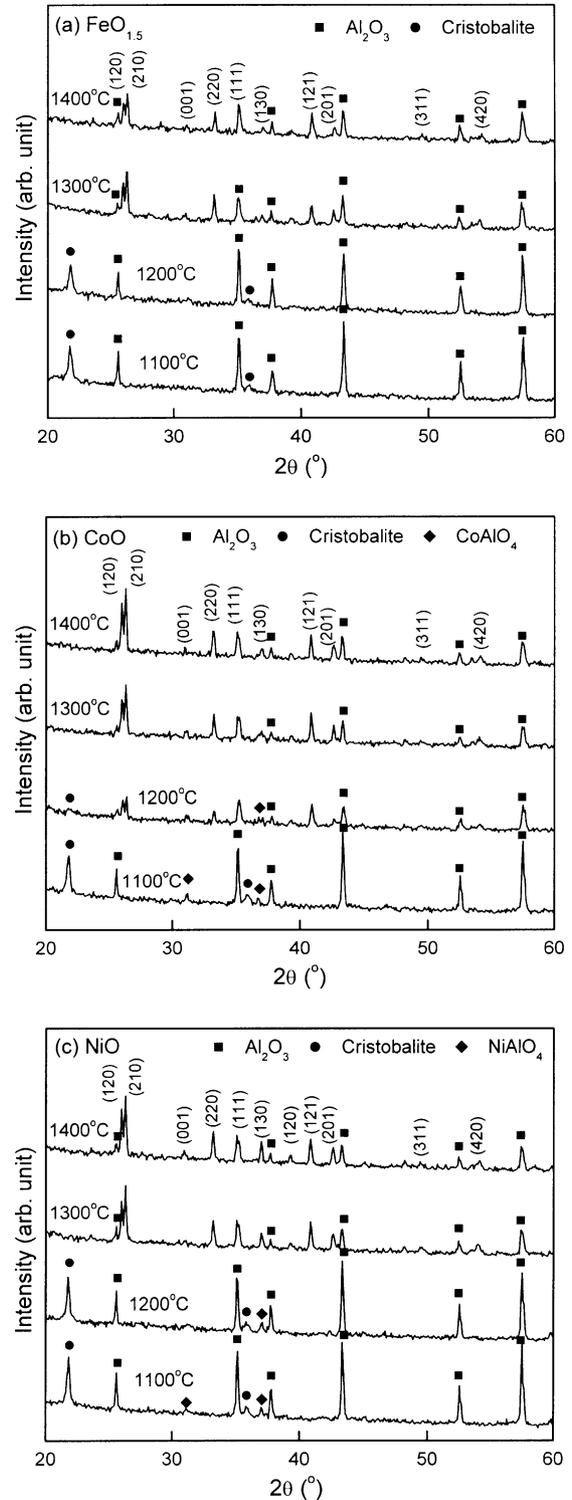
Fig. 4. XRD pattern of the unmilled mixtures doped with the transition metal oxides sintered at different temperatures.
