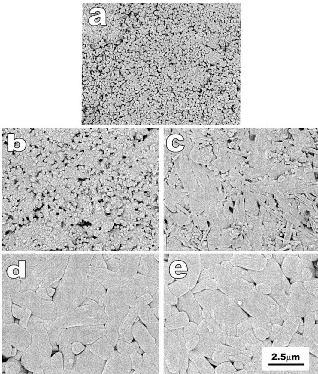
Fig. 7. SEM images of the NiO-doped mixture sintered at different temperatures: (a) 1000 °C, (b) 1100 °C, (c) 1200 °C, (d) 1300 °C and (e) 1400 °C.
