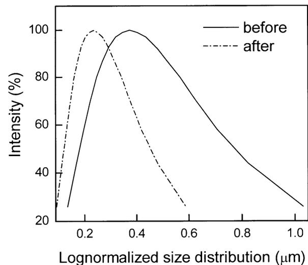
Fig. 11. Particle size distribution of the mixture of  $\text{Al}_2\text{O}_3$  and silica before and after the high-energy ball milling.
