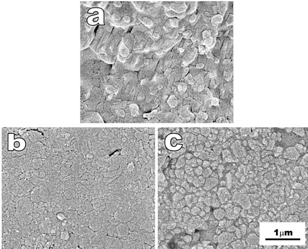
Fig. 10. SEM images of the unmilled mixtures sintered at 1400 °C: (a)  $\text{FeO}_{1.5}$ , (b) CoO and (c) NiO.
